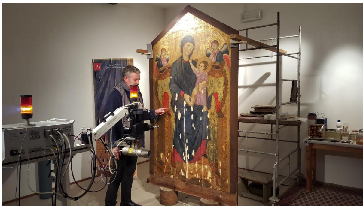
Fig. 1 Portable non-invasive x-ray fluorescence analysis of Cimabue's Maestà , a panel painting from the late 13th century from the Church of Santa Maria dei Servi in Bologna.
